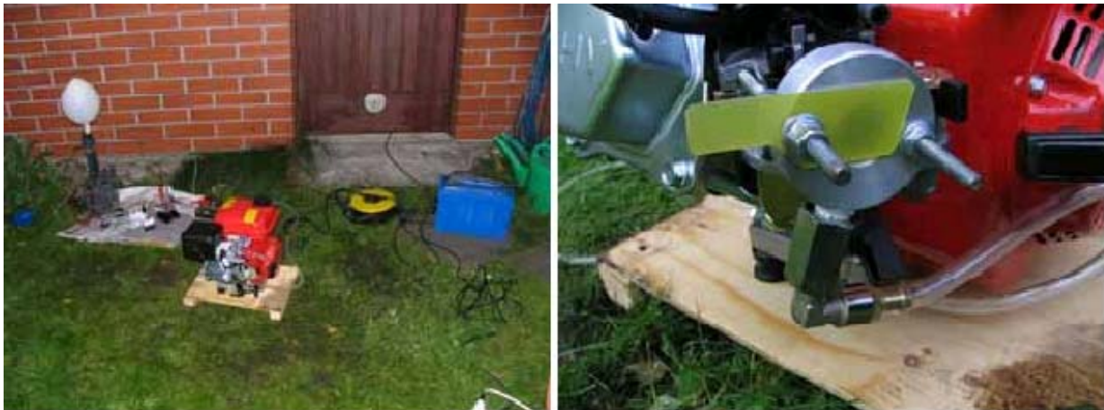
Figure 14. 6.5hp 200cc 4-stroke running on electrolytic gas
